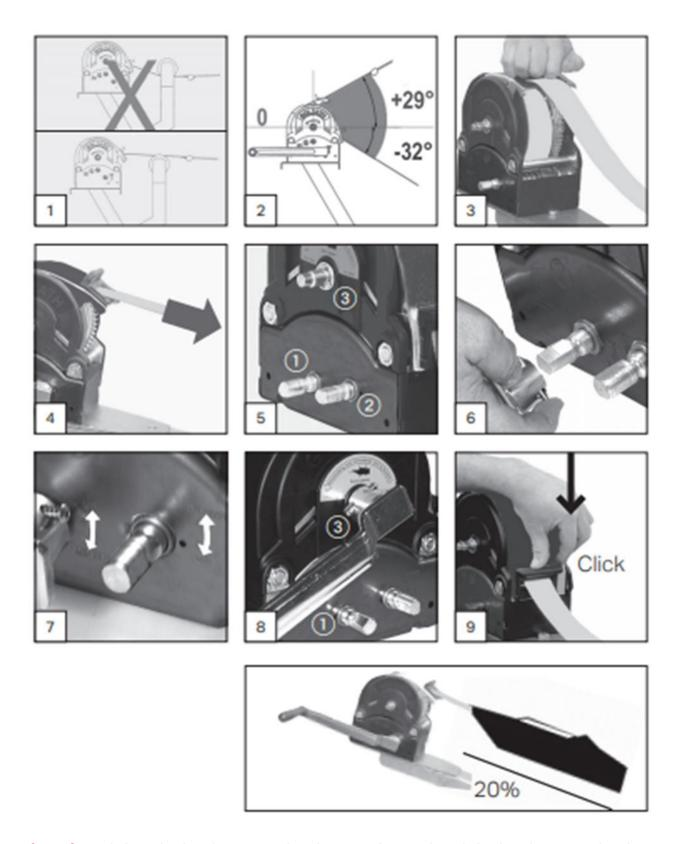
If it is found that the hauling strap has been tightened and the hook cannot be disengaged, it is possible to release the ratchet mechanism pawl by VERY CAREFULLY PUSHING A SUITABLE IMPLEMENT (E.G. SCREWDRIVER) AGAINST THE PAWL.
